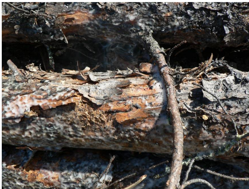
Figure 3. Ignition of a gel covered deck where a cone has fallen between the logs and into the unprotected interior of the deck – smoke is showing in the center of the photo.
