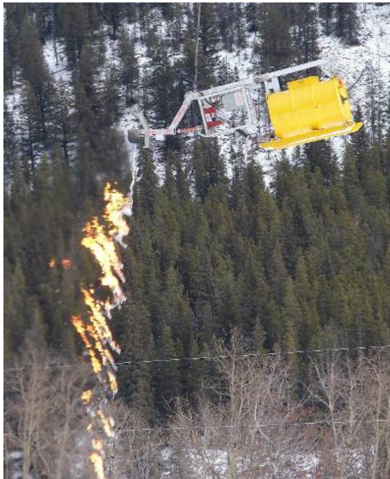
Figure 3. Torch operation showing desirable performance.
