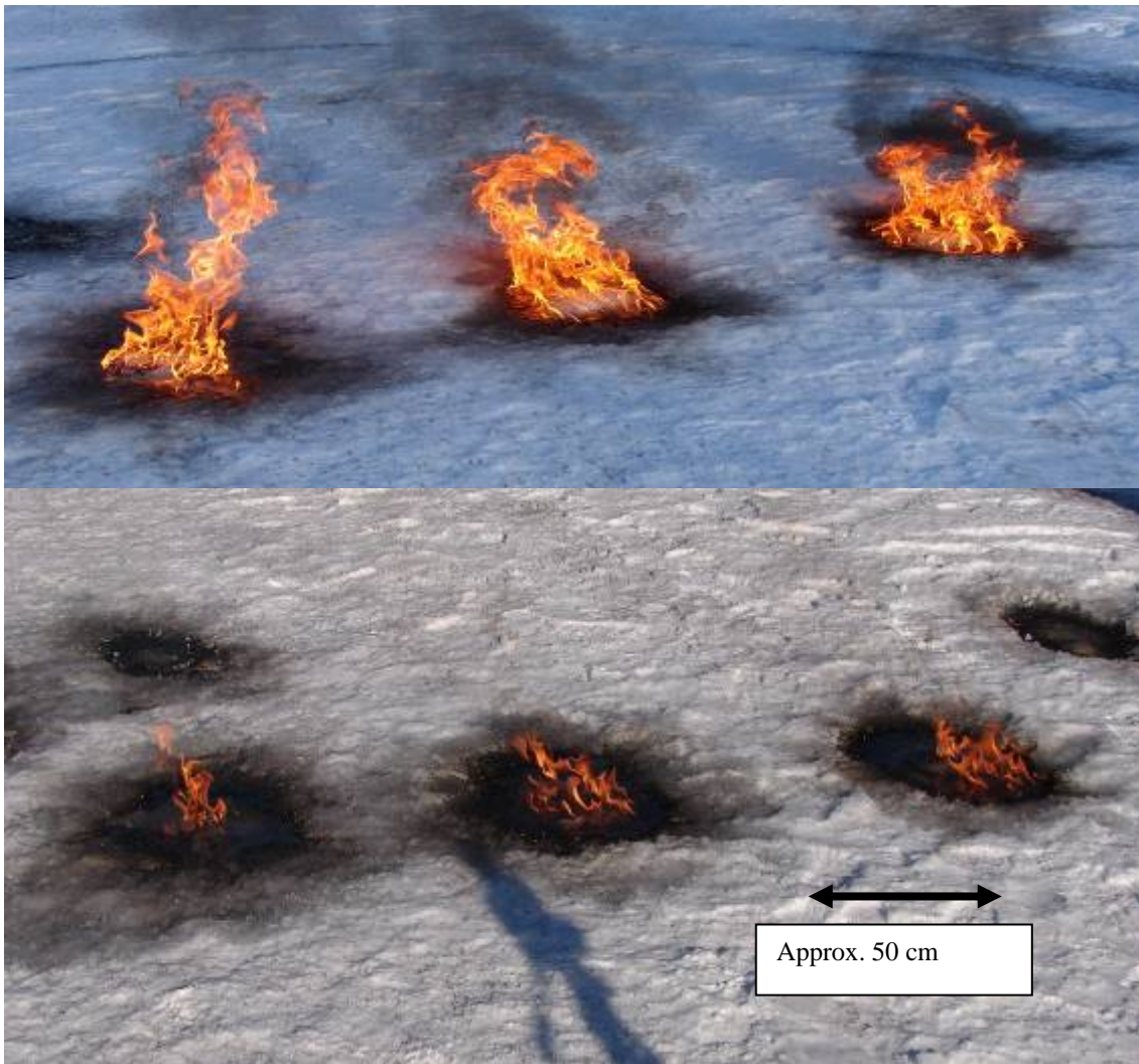
Figure 4. Ground ignition tests – 300 ml samples. Top – after ignition. Bottom – almost burned down. Left = Unleaded gasoline, Center = Jet B/unleaded gasoline (50-50 mix), Right = Jet B + 10% gasoline.
