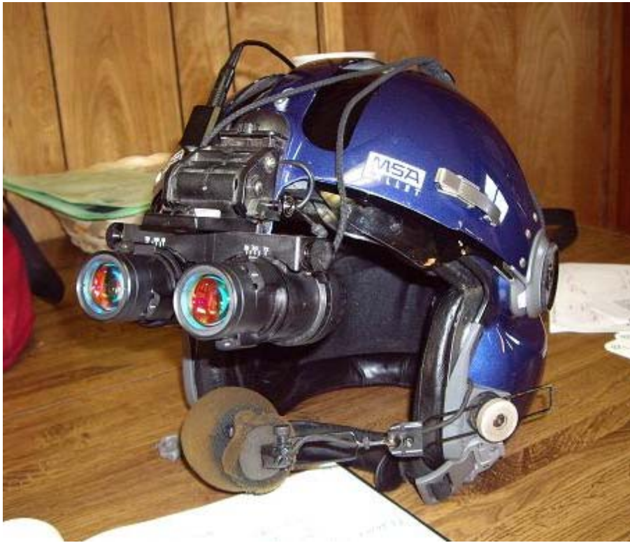
Figure 3. ITT F4949 NVG attached to flight helmet. Battery pack attached to rear of helmet (4 AA).
