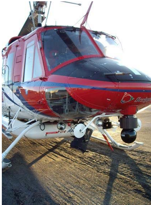
Figure 8. FLIR mounting, Night Sun Search light, Standard searchlight – Note Standard Searchlight is all that is needed for the NVG. Night Sun is too bright in most situations.
