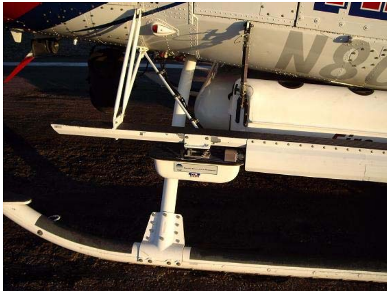
Figure 5. Microwave system for transmitting live image data to ICP (FLIR usually). Also receives data updates from the ground.
