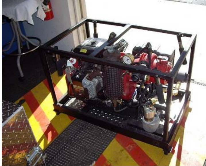
Figure 1. Prototype Remote Start Pump: note priming motor on the right.
