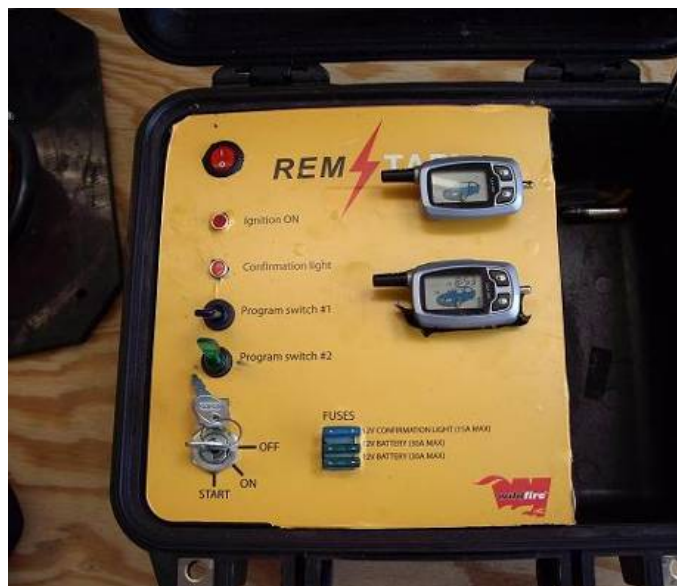
Figure 2. Wildfire RemStart Control Box Prototype – Initial technology based on remote car starter.
