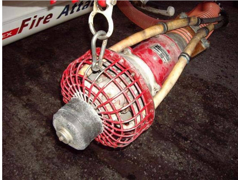
Figure 7. Hydraulic pump on tank snorkel can fill the tank in under 10 seconds.
